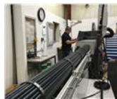
The LNS Tryton bar feeder excels at handling smaller diameter barstock, accepting bar lengths as long as 12 feet with diameters of 0.039 to 0.500 inch.
